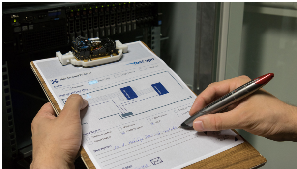
Figure 1. Maintenance Form Filling Application: Our smart form system supports maintenance workers to create error reports faster by providing real-time status information for network machines on the paper itself using novel printed electronics.
