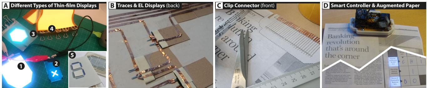
Figure 13. We considered several thin-film display technologies: cut (A1) & stenciled EL foils (A2), printed EL segments [46] (A3), elastomeric ELastoLite Panels® (A4) end printed EC SSDs [67] (A5). Finally, we used cut & stenciled EL foils in fast iterations. To realize paper traces we used combinations of copper (B) as well conductive tape with conductive ink (C). As a result, we came up with a 27 pin connector (C) for our smart clip (D).
