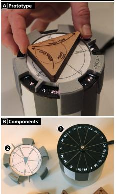
Figure 1: ScaleDial (A) teaches music theory by transferring musical geometry to physical representations. Scale caps (B2) and triad tokens (B3) can be arranged on top of an interactive scale cylinder (B1).
