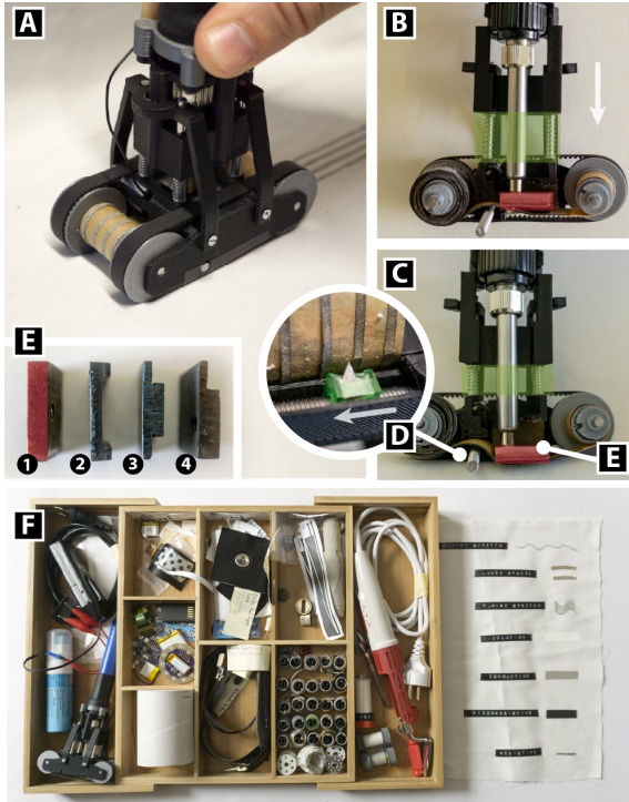
Figure 1: Rapid Iron-On User Interfaces constitute a new fabrication approach for textile prototypes. By using a handheld ironing tool for applying adhesive functional tapes and patches, the designer can create rich interactive functionality in a fast and intuitive sketching-like manner.
