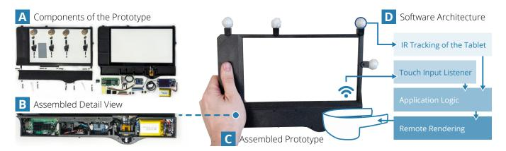
Figure 2: Our hardware setup consists of a Raspberry Pi Zero 2 W, a 10" transparent capacitive touch panel, and a battery. We installed these components in a custom, 3D-printed case and attached reflective tracking markers. Both the pose data of the tracked interaction panel and touch events are sent to the application. We use remote rendering to stream content to the HMD, which then displays the holograms, e.g., on the panel.
