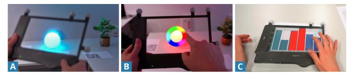
Figure 5: CleAR Sight allows configuring smart devices such as smart bulbs (A) and directly seeing the effects, e.g., color changes (B). We can show interactive 2D content on the panel. For example, when used as an overlay, the tablet allows selection in printed charts; selected data points are highlighted (C).
