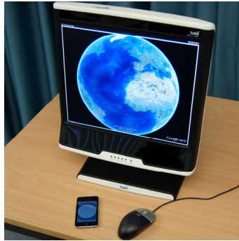
Figure 2: General demo setup – a Tobii T60 eye tracker to collect gaze data and a mobile touchscreen.
