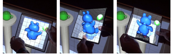
Figure 7. Mobile fish tank windows serve as physical proxies for virtual objects that users can inspect by moving/rotating the display. The backside of an object can be inspected by flipping the window.
