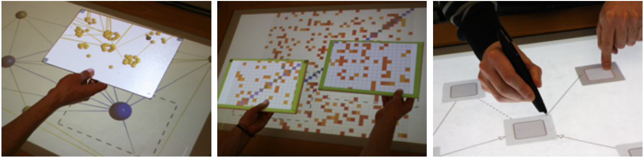
(a) Semantic zooming of node-link diagrams by lifting/lowering a tangible view [13]. (b) Tangible views applied to compare different parts of a matrix visualization [13]. (c) Manipulating node-link diagrams by using multi-touch and pen input [3].
