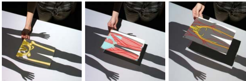
Figure 1: Exploration of a layered information space with the paper lens. Depending on the height of the paper lens, different layers of information are displayed, i.e. skeleton (left), muscles (middle) and nerves (right).
