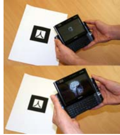
Figure 4: UMPC Lens Setup. The build-in UMPC camera tracks a printed marker (ARTag) and displays slices of a 3D volume depending on the distance to the marker.
