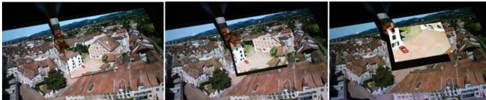
Figure 6 Exploration of a zoomable information space with the paper lens. Depending on the height of the paper lens, the level of detail on the lens is changed from small (left) to large (right).
